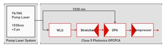
Basic schematic set-up comprising: Yb-based pump laser, White Light Generation (WLG) to generate a broad-band signal pulse, stretcher to optimize bandwidth and temporal overlap between signal and pump pulse, optical parametric amplifier (OPA) to amplify signal pulse, compressor to compress amplified signal pulse to its Fourier transform limit.
